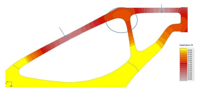
**Picture comments:** There are distinct split points where the arrows are placed. It looks good but the angle of the metal front is too blunt, it should be pointed. The metal front should look like an arrow with a sharp edge. The inner angle of the arrow should be small to make sure that there is no risk that the melt divides in small islands.
