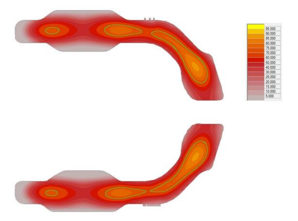
**Picture comments:** This is an example of a casting where there is serious splitting of the melt. This will cause shrinkage defects. Using some simple design rules when designing the casting will result in a more directional solidification and also define distinct splitting points.
