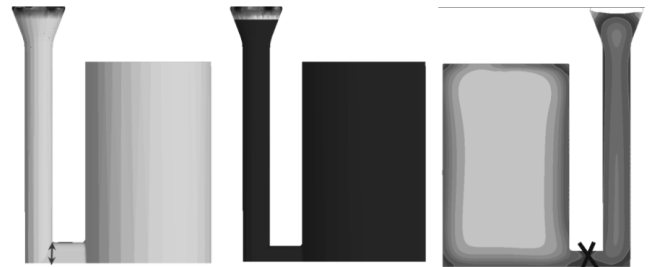
Fig. 7. The feeding from runner system.
