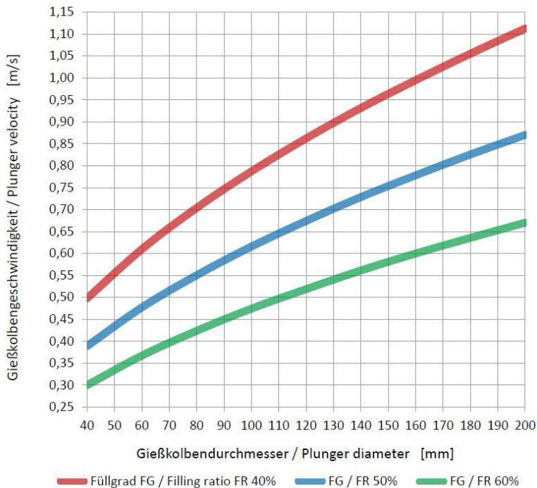
Fig. 5: v_{krit} diagram for estimating suitable casting piston speeds v_k .
