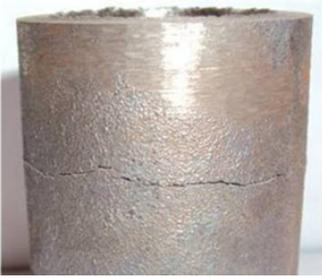
**Figure 6:** Hot Crack [12]
